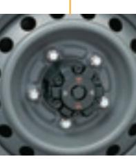
Optional Dual Mode Automatic Locking Hub lets you lock the front wheels and switch between 2WD and 4WD from the driver's seat.
